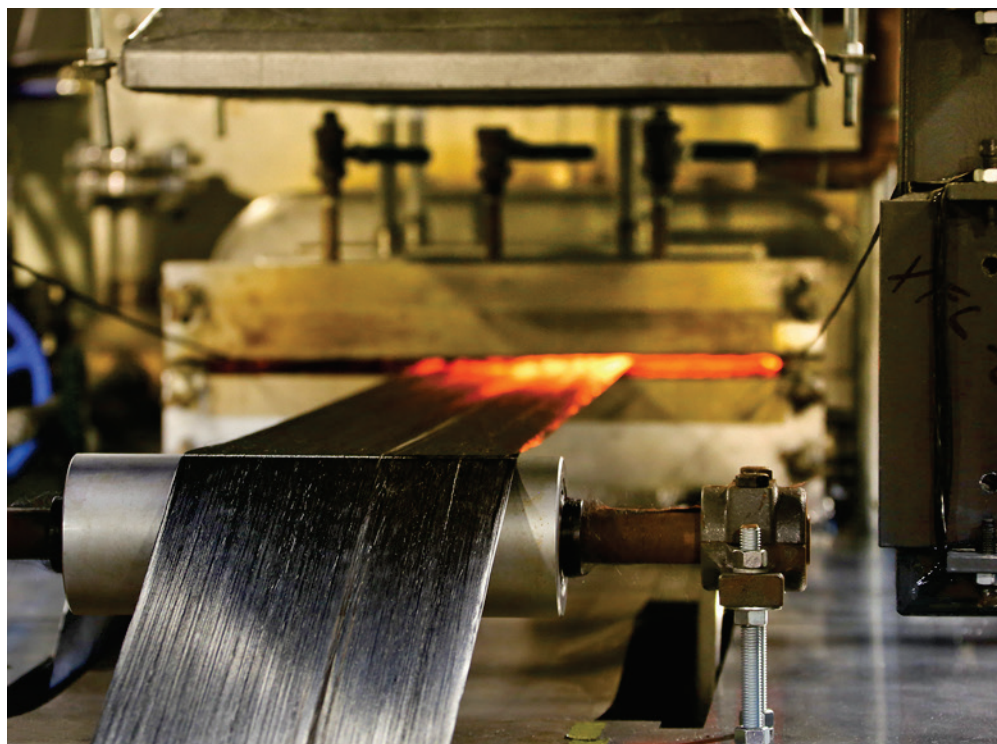
Fig. 5.2. Production of lower cost carbon fiber at the Carbon Fiber Technology Facility.
